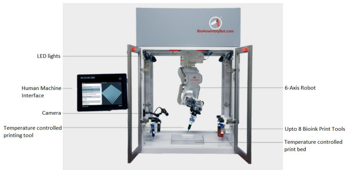
Fig. 3 Components of the BioAssemblyBot® [12]
