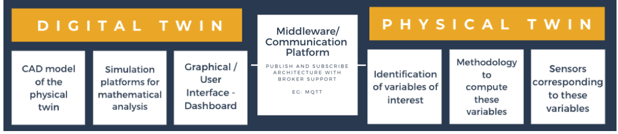
Figure 7: Illustrates the concept of Digital Twins through a bending beam test bench [19]
